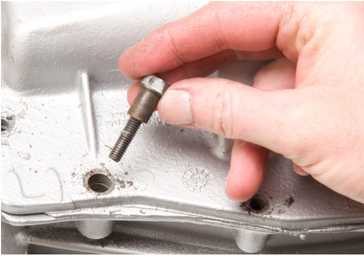
Remove the top cover bolts, noting that two of them have shoulders to center the plate. Handle with care, as the top bolts are thin and can break and/or strip easily.
