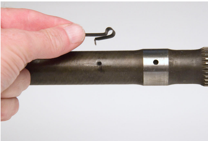
The two holes are not far apart. Note that the shaft is thicker where the gear was located. You will need to make a shim from steel and/or brass to put under the gear in its new location.
