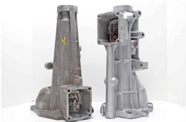
The S10 tail housing is on the left. Note that the shifter box is near the front (gearbox end) of the housing, while the Camaro tail housing at right locates the shifter at the very back. Before you re-install the S10 tail housing, replace the rear seal and the tail shaft bushing (if available). The rear transmission mount is in the same place on both housings, but differs from a T10/Muncie, so you may have to move your chassis mount.
