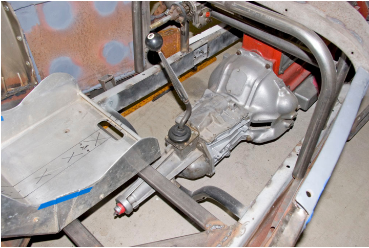
Here's the box mocked up in our 1927 track roadster. Note the shifter location in relation to the seat – the Camaro tail housing wouldn't have fit. Neither would conventional side-shifter boxes like T10s and Muncies. The hybrid S10/Camaro T-5 is a great solution at a bargain price for rodders in need of a fifth gear for cruising.
