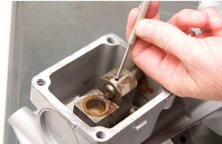
First we take off the shifter, and then drive out the pin that holds the shift finger to the top plate shaft. Drive the pin all the way out, or it will come back to haunt you when reassembling the unit. Underneath the finger is a spring and a detent ball, so don't drop them when you slide the finger off the shaft. Bag the pin, spring, finger and ball to keep them secure.
