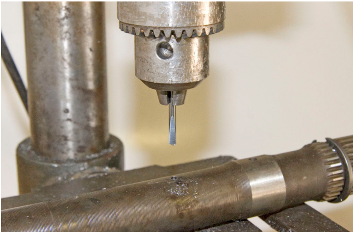
Drill a new hole to the depth and diameter of the clip pin. After rounding off two titanium drill bits, we decided to order a 1/8-inch solid-carbide spade-tip drill bit from Enco ( use-enco.com ) for $7.95, and it worked like a charm. Don't drill any deeper than necessary – it weakens the shaft.
