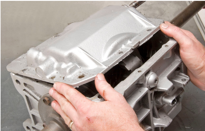
Remove the top by pushing away from you using your thumbs before lifting the lid off.
