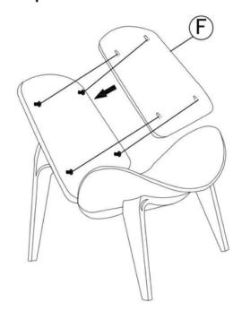
Use the four holes on the back of F to align the four screws on E and hang them up
