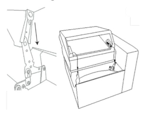
Lay the back rest face down and allign the male and female slots.
