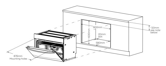
NOTE: If a powerpoint is fitted it must be accessible with the appliance installed.
