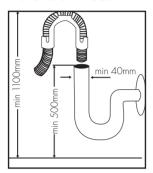
The water drain hose can be connected either directly to the water drain hole or to the sink outlet spigot. Using a hose hook (if available), the water can be drained directly into the sink by positioning the hose hook over the edge of the sink.
