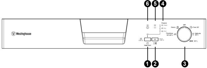
Rotate the Program Selection Knob (3) to switch the machine on and select a suitable program for your dishes.
