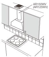
Optional carbon filters(AR610CF) diminish cooking odours in the recirculated air. Depending on the frequency of use and the type of cooking, the expected life of carbon filters is 3 months. Using carbon filters will reduce the airflow of the rangehood.
