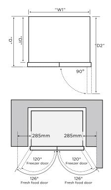
When positioned in a corner area, spacing of at least 285mm on the hinge side will allow the doors to open enough to enable the removal of bins and shelves.
