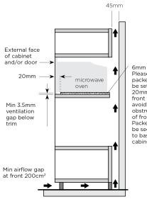
6mm packer Please note packer must be set back 20mm from front trim to avoid obstruction of front vent. Packer must be secured to base of cabinet.
