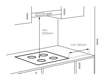
NOTE: The clearance must meet or exceed the minimum recommended for both the rangehood and cooktop.
