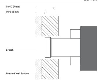
Firmly screw Spindle into the Breach.
