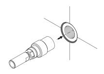
2 Fit Fibre Washer around the Spindle and the the Spindle and then firmly fasten the Bonnet onto the Spindle using a spanner.
