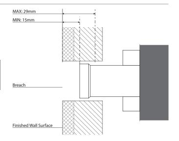
Firmly screw Spindle into the Breach.
