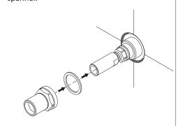
Fit O-Ring to the groove in the rear of the Dress Plate.
