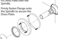
Fit Handle to Spindle and fasten with the Grub Screw using the Allen Key provided.
