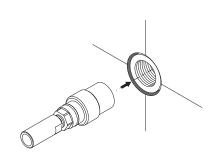
Fit Fibre Washer around 2 Fit Fibre washed then the Spindle and then firmly fasten the Bonnet onto the Spindle using a spanner.
