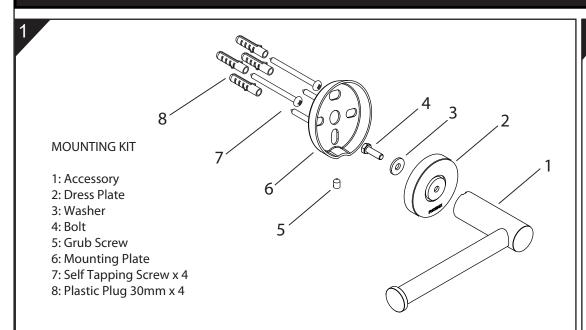
Place fixing plate where accessory is to be mounted. Mark center position of slotted holes.
