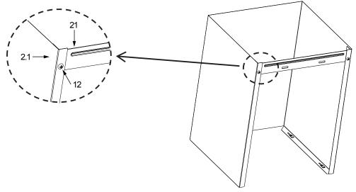
• Slightly widen the two sides of the flue and hook them onto the hood body, making sure that they are well seated.
