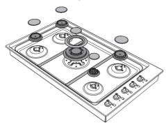
3. Replace the burner nozzles using a 7 mm socket wrench according to the gas to be used (see "Burner and nozzle characteristics tables").
