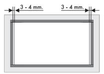
2. Make the seal stick to the edge around the hole cut in the worktop, using a slight pressure; front and rear sides of the seal must brush against the hole.
