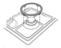
The ring must be placed under the hob grid as shown in the picture above.
