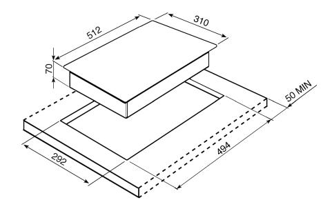
**finish** stainless steel, cast-iron trivet **size** 310mmW x 70mmH x 512mmD
