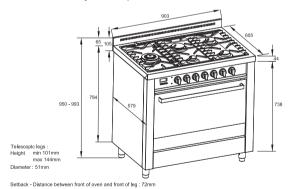
Total depth of the unit when oven door is open: 1012mm
