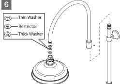
Ensure restrictor and washers are installled correctly. Screw Shower Rose to Shower Arm. Tighten firmly. Insert Shower Arm Assembly onto Shower Rail Tube. Tighten grub screw firmly.
