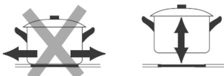
For maximum efficiency the pot should be the same size as the cooking zone, with the pan centred on the cooking zone. Pots with a diameter larger than the cooking zone should not be used.
