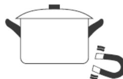
Move a magnet towards the base of the pan. If it is attracted, the pan is suitable for induction. If you do not have a magnet, put some water in the pan you want to check, and then if **U** does not flash in the display and the water is heating, the pan is suitable.
