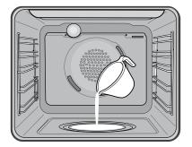
Add 150ml of water into the cavity of the oven. Fill the cavity well with water only when the oven is cold.
