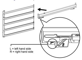
The shaded wires indicate the wire the slide can be mounted on. Fit slide rear clips to the rear of wire at an angle as shown below.
