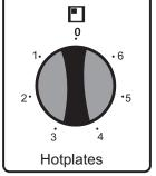
1........Keeping hot location 2-3......Heating locations at low heat 4-5-6..Cooking - roasting and boiling locations
