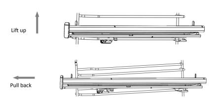
One hand finger is pressed the button of the front clip, another hand holds the telescopic runner front end to lift up first , then pull it back . It's easy to remove .
