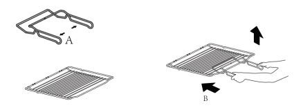
Please use both hands to hold the holding parts(A). Then move it along the direction B until it reaches the position like the picture showing. Finally, lift the racks up to move.
