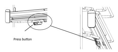
Press the front clip button to remove the boss off the outer wire.
