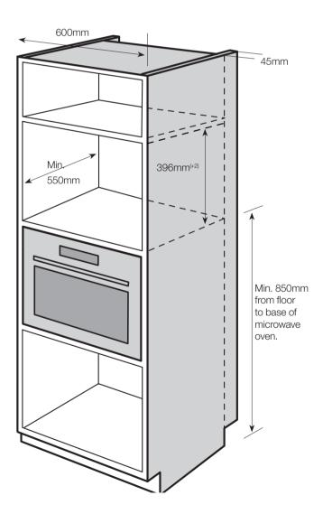
A 45mm ventilation gap must be left between the built-in cabinetry and wall with no back panelling on the cabinet housing the microwave oven. A ventilation gap of min. 3.5mm must be left between the bottom of the front trim and adjacent shelf/cupboard).
