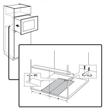
5. Open the door and fix the appliance to the cabinet with a screw.
