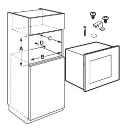
3. Put the template on the bottom of the cabinet and mark the spots for screws. Remove the template and fix the bracket with the screws.
