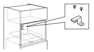
4. Install the appliance. Make sure the bracket locks the back of the appliance.
