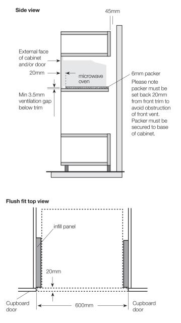
Infill panels are recessed 20mm from the external cabinet door to accommodate flush fit.
