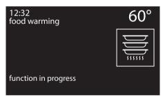
While the function is in progress, it is possible to set a timer for a maximum of 4 hours (see "Timer during a function"), a warming duration (see "Timed cooking") or a delayed warming (see "Programmed cooking").
