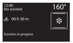
4. At the end of the cooking cycle, "function ended" is shown on the display and a buzzer will sound that can be deactivated by pressing or turning one of the two knobs or opening the door.
