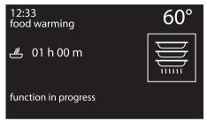
At the end of the function, "function ended" is shown on the display and a buzzer will sound that can be deactivated by pressing or turning one of the two knobs or opening the door.
