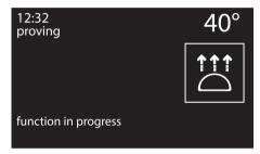
While the function is in progress, it is possible to set a timer for a maximum of 4 hours (see "Timer during a function"), a proving duration (see "Timed cooking") or delayed proving (see "Programmed cooking"). 7. Press the control knob to make the desired changes.
