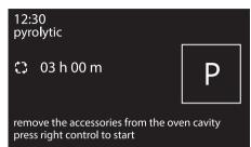
4. Press the control knob to start the pyrolytic cycle.
