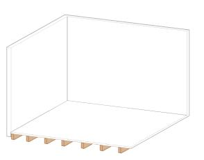
STEP 1: when walls are sheeted and structural floorboards installed, mark a slightly larger area than the Domus shower floor being installed (ex. for a 900x1600mm shower floor mark an area of 910x1610mm, so 10mm more length and width) and set the plumbing device (100mm puddle flange or smart-pan).
