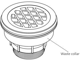
2) It is mandatory that the smart pan lid has to be cut to waste collar size and it is not to be removed. The lid support is essential. Failure to follow this instruction will void the warranty for the Domus shower floor.
