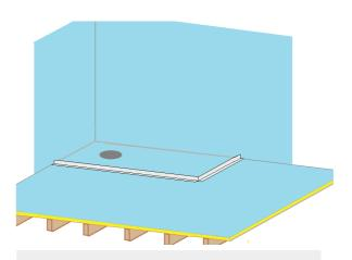
STEP 2: waterproof the bathroom floor / walls as AS AU3740 and install a PVC angle to separate the bathroom area to be screeded from the Domus shower floor area (not scredeed)
