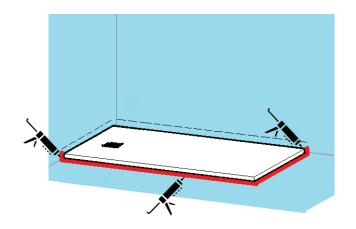
Seal the edges of the Domus shower floor to the waterproof membrane with a waterresistant polyurethane sealant (see point 6 for the sealant recommended). It is advisable not to seal the Domus shower floor to the waterproofing membrane on the
