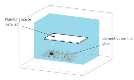
Spread flexible cement based tile glue (see point 6 for the glue recommended) with a 12mm notched trowel, install the plumbing waste supplied on the Domus shower floor, then put the Shower Floor in place.
