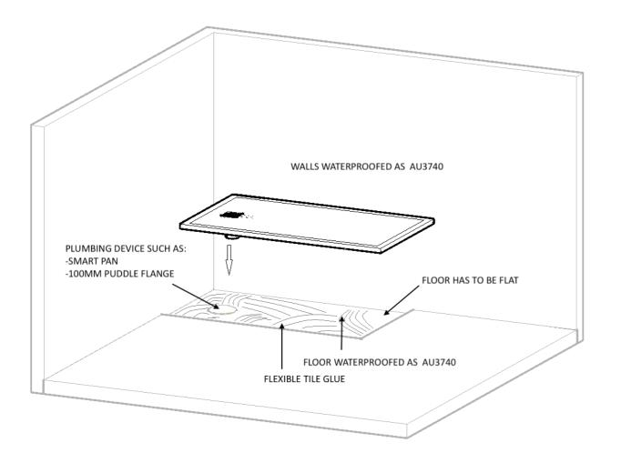
The image above represent the ordinary installation method of a Domus shower floor: flat floor, plumbing device installed, tile glue in place.
