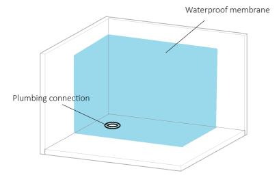
After\_installing the plumbing device according to the Domus shower floor waste position, the whole shower area must be waterproofed according to AS AU3740.
