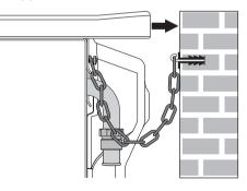
The chain length must be as short as practicable to avoid appliance tilting forward and also diagonal to avoid appliance moving sideways.
