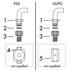
Carefully screw the connector  ${\bf 3}$  to the appliance's gas connector  ${\bf 1}$  (1/2" thread BSP), placing the supplied seal  ${\bf 2}$  between them.
