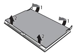
Some models have an intermediate glass pane. Remove the intermediate glass pane by lifting it upwards.
