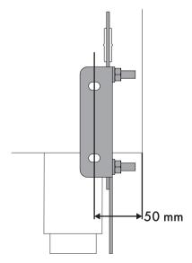
Move the bracket onto the wall and mark the position of the holes to be drilled in the wall.
