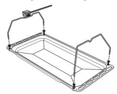
Prepare the rotisserie rod with the food using the rotisserie rod provided. The clip forks can be tightened using the fastening screws.
