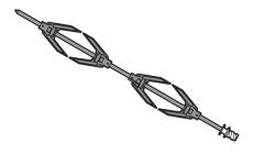
Once you have prepared the rotisserie rod, place it on the supports. Insert the tip of the rod in the housing of the mechanism on the left-hand support until it stops.
