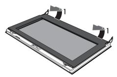
4. Pull the internal glazing pane from the front strip (2) to remove it from the door.
