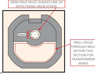
NOTE: FOR HORIZONTAL INSTALLATION ROTATE THE DRILLING PATTERN 90° WITH SINGLE HOLE LINING UP WITH FIXING SCREW HOLE.
