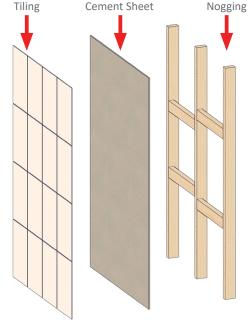
Consider utilizing noggings with 18mm construction plywood to cover a larger area if the precise position cannot be determined at the beginning of the job.
