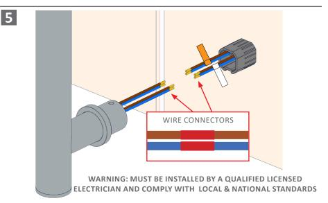
Place Towel Rail onto the wall brackets, connecting correct wires and feeding them through the holes where possible.
