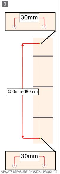
To adjust bottom pillar use a screwdriver to loosen. Adjust to desired vertical location and tighten
