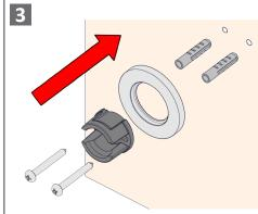
To adjust the bottom pillar, use the supplied Allen key to loosen it as shown. Move it to the required distance and tighten it securely.
