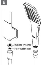
Insert Rubber Washer and Flow Restrictor as shown into Shower Hose. Screw Shower Hose to Hand Shower and Shower Rail
