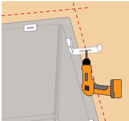
Drill pilot holes around the sink perimeter, depending on the fasteners being used.
