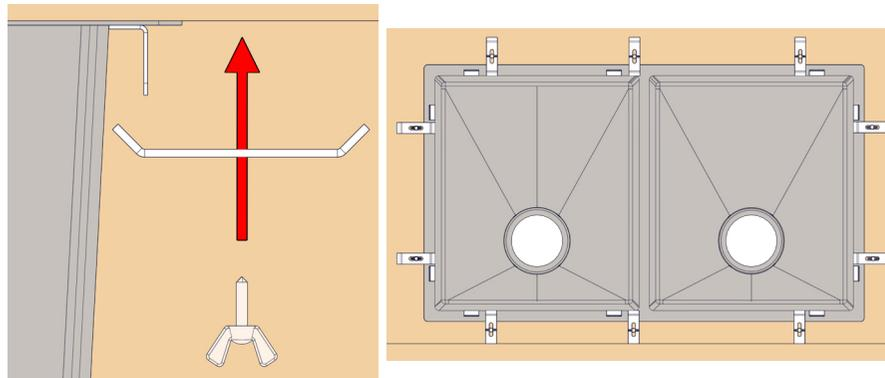
Fasten the Sink Clips using the pilot holes all around the bottom of the sink.
