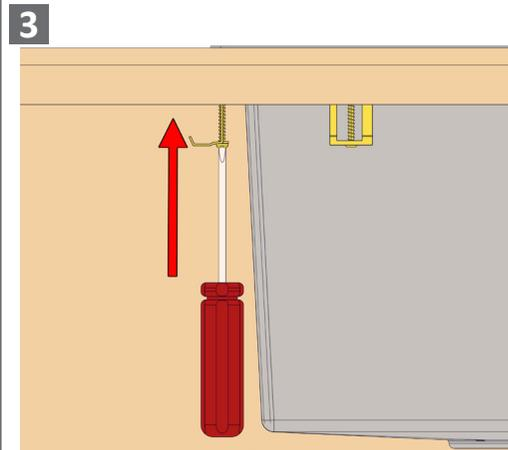
Tighten the Sink Clips using a screwdriver
