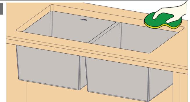
Clean up around edges and remove any excess sealant where possible.
