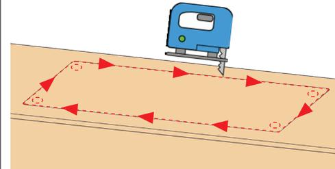
Using a suitable tool, cut a hole in the in the benchtop along the marked out lines.
