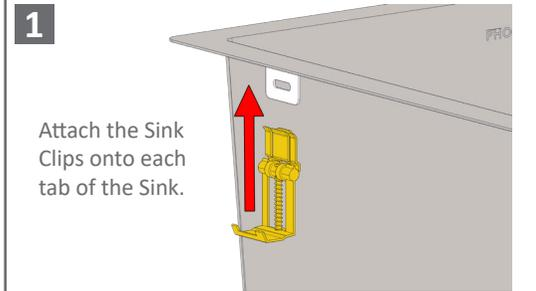
Attach the Sink Clips onto each tab of the Sink.
