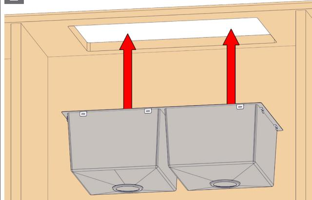
Place the Sink under the benchtop, aligning it with the bench cutout.
