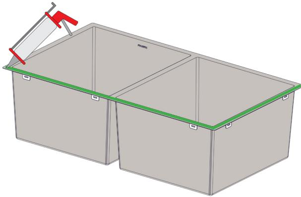
Apply adhesive sealant on the top sink surface
