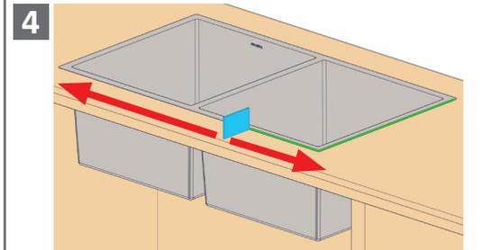
Carefully trim, or use a card to remove any excess sealant around the edges of the sink.
