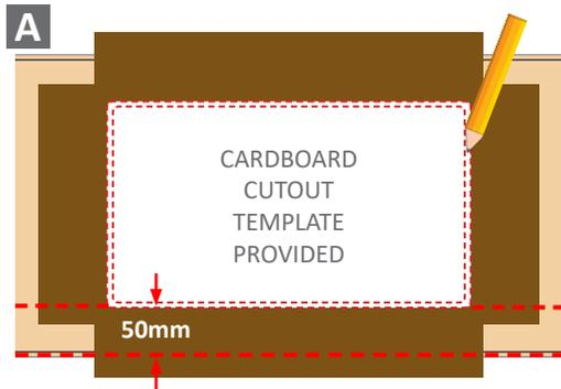
Using the sink template provided, draw a cutting line on the worktop.
