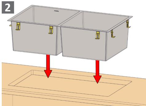
Carefully drop the sink into the cutout hole in the benchtop.
