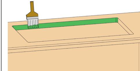
Seal the cut surfaces using caulk if required.
