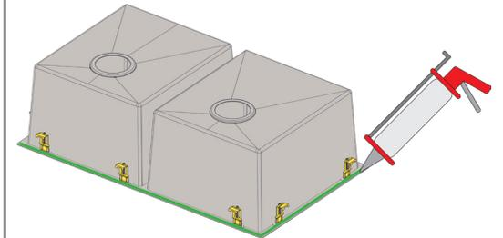
Apply adhesive sealant under the sink to ensure a tight seal.
