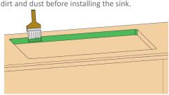
Seal the cut surfaces using caulk if required.
