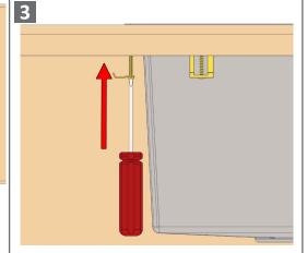
Tighten the Sink Clips using a screwdriver
