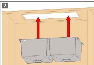
Place the Sink under the benchtop, aligning it with the bench cutout.
