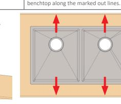
Carefully drop the sink into the cutout hole in the benchtop.
