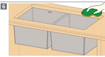
Clean up around edges and remove any excess sealant where possible.
