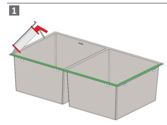
Apply adhesive sealant on the top sink surface
