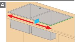
Carefully trim, or use a card to remove any excess sealant around the edges of the sink.
