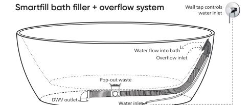
Smartfill has two elements of backflow prevention built in to the device. Smartfill passes AS2845:2:1996 for backflow prevention with included air gap and also has a dual check valve (DualCV). WM Cert 23422.
