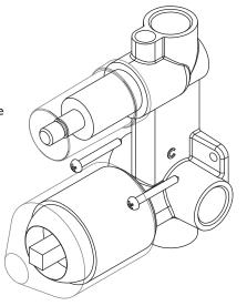
Cut a 40mm hole and a 54mm hole in cement sheet and tiles, 68mm apart, as shown.
