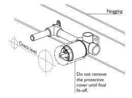
Connect hot and cold water supply, as shown.
