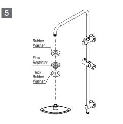
Insert washers and flow restrictor as shown into Shower Rose. Screw Shower Rose to arm with care, ensuring the flow restrictor is not damaged.
