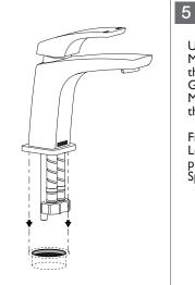
Underneath the Mounting Hole, feed the Rubber Mounting Gasket then the Mounting Plate onto the Threaded Rod.
