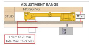
Range from the Nogging face to the Stud Face is 32mm as shown.
