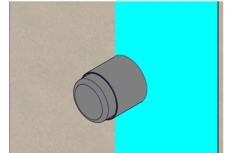
**4** After Tiling use Knife to Trim Waterproofing Sleeve flush to Tile face.
