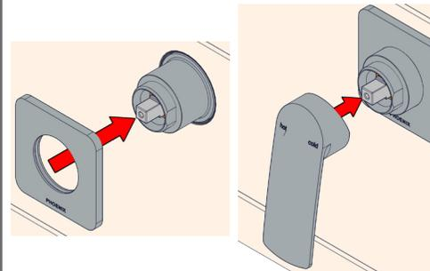
**6** Tighten Grub Screw and push in Cap to secure handle.
