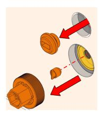
Remove Test Caps with a flat head screwdriver or spanner.
