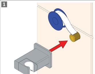
Apply teflon to wall thread and screw on Mounting Bracket.
