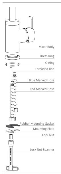
Cut a mounting hole 35mm in diameter. There must be a minimum 12mm width of flat surface around the hole.
