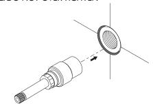
Fit Fibre Washer around the Cartridge and then firmly fasten the Bonnet onto the Spindle using a spanner.
