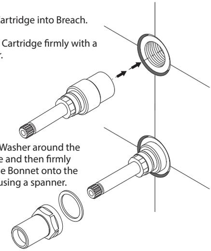
Fit Fibre Washer around the Cartridge and then firmly fasten the Bonnet onto the Spindle using a spanner.
