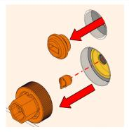
Remove Test Caps with a flat head screwdriver or spanner.
