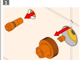
Remove Test Caps with a flat head screwdriver or spanner.
