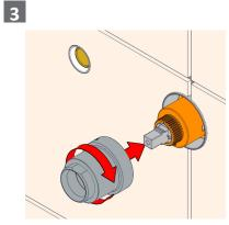
Firmly fasten Cartridge Sleeve to Mixer Body using a shifting spanner.
