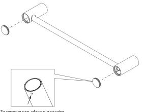
To remove cap, place pin or wire into hole shown and push firmly
