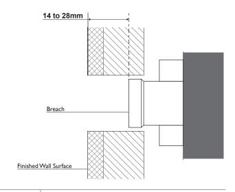
Firmly screw Spindle into the Breach.
