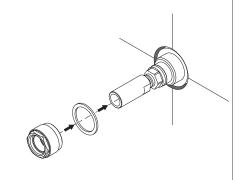
Fit O-Ring to the groove in the rear of the Dress Plate.
