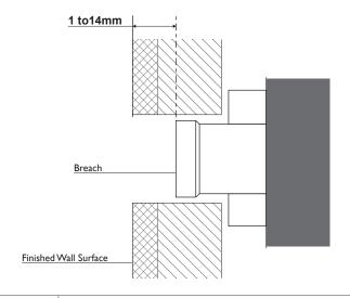
Firmly screw Spindle into the Breach.
